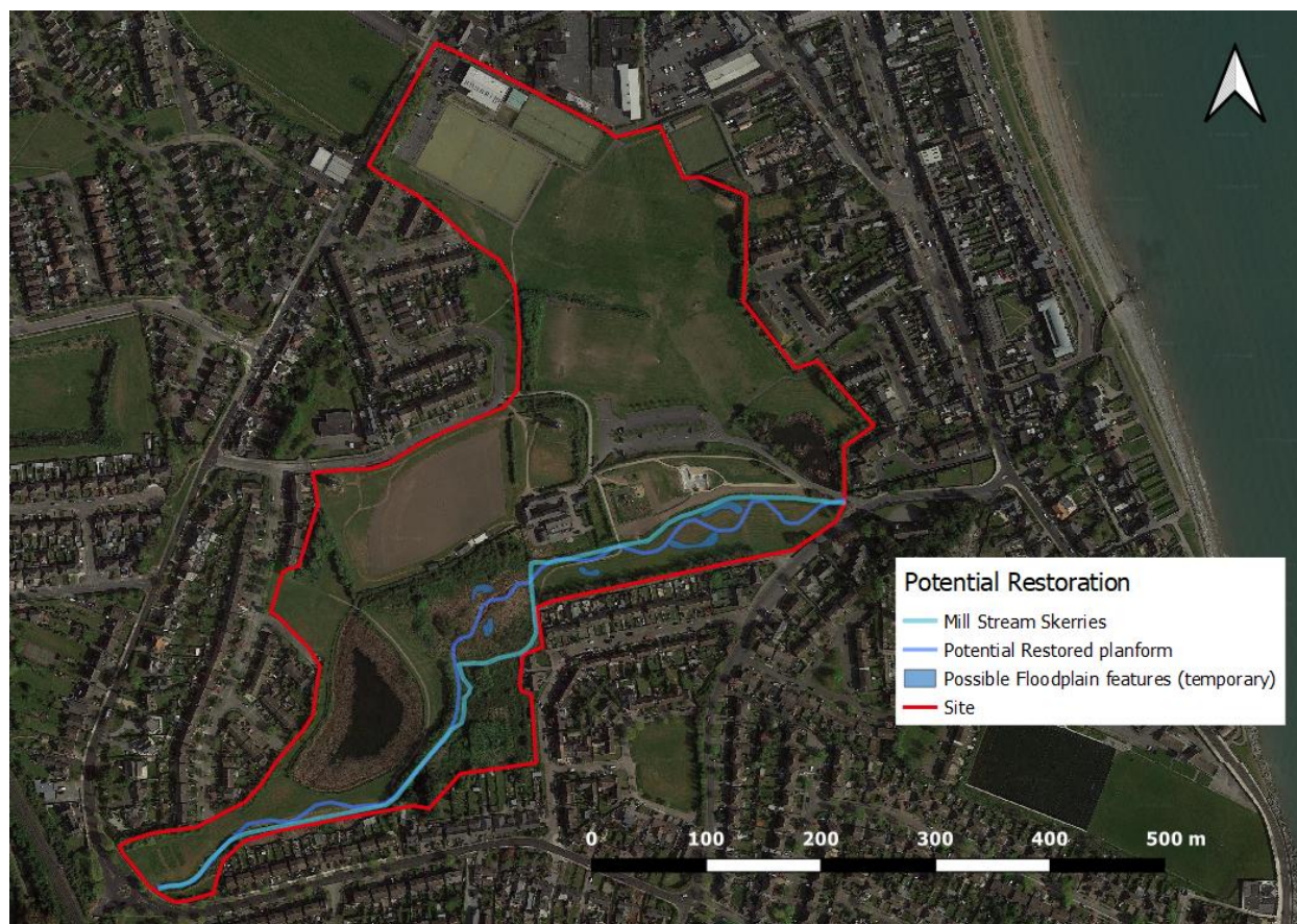
Figure 15 Conceptual diagram of a re-naturalized river section through the Town Parks
