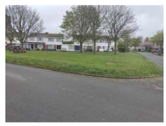
Flooding has been reported in Churchfield Close, and here in the green areas (such as L) the ground level could be dropped to allow gravity flow into a bioretention area for flood water storage and infiltration to ground. Maximum flood depth of 150mm during storm events.
