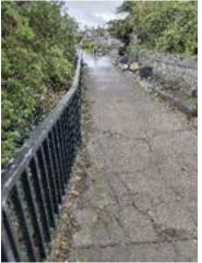
Just inside the cemetery gate there is a very small area of ground behind the railing (L) which could potentially afford a 30cm wide swale for modest rainwater storage and conveyance. The biggest advantage here is not so much flood water storage per se, but removal of water from the pathway in wet conditions, if this is a problem.
