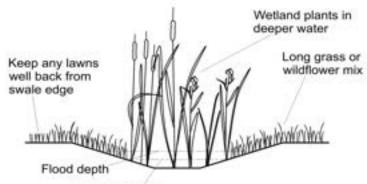
Section through planted wet swale (L). In essence, a wider version of this set-up serves as a stormwater wetland. (Image: FHWS)
